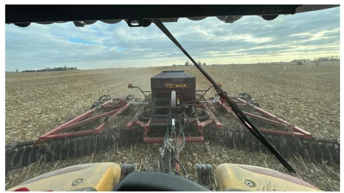
Air seeders mounted on vertical tillage tools are proving to be a popular and effective way to plant cover crops in the Lower Cedar Watershed.
