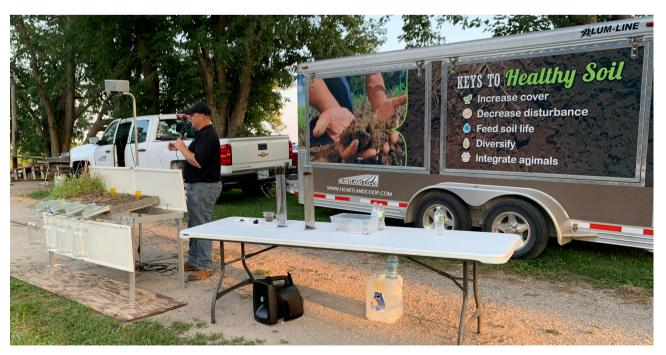
J.D. Hollingsworth uses a rainfall simulator to demonstrate how different management techniques affect soil infiltration and runoff. .
